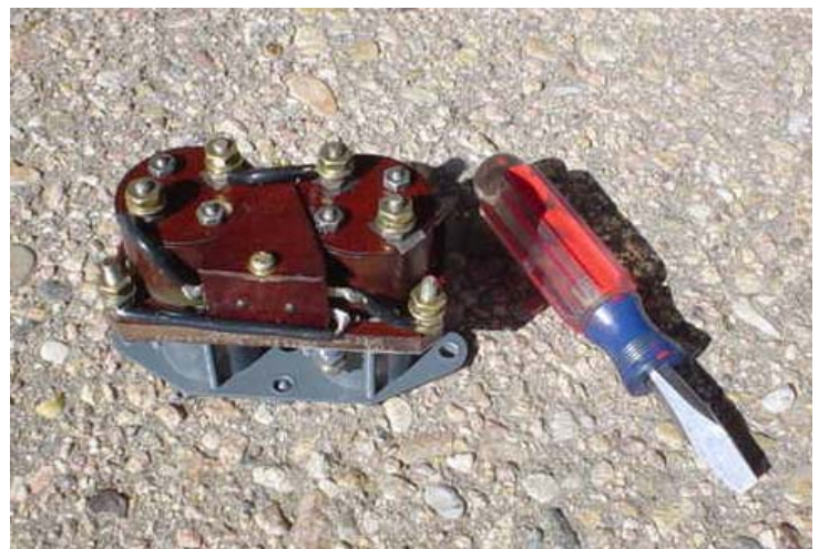
New brake relay before installation
