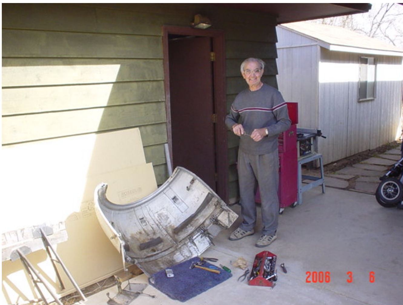
Joseph Brexa works on the “mystery part”—fixing the cowl flap bushings
