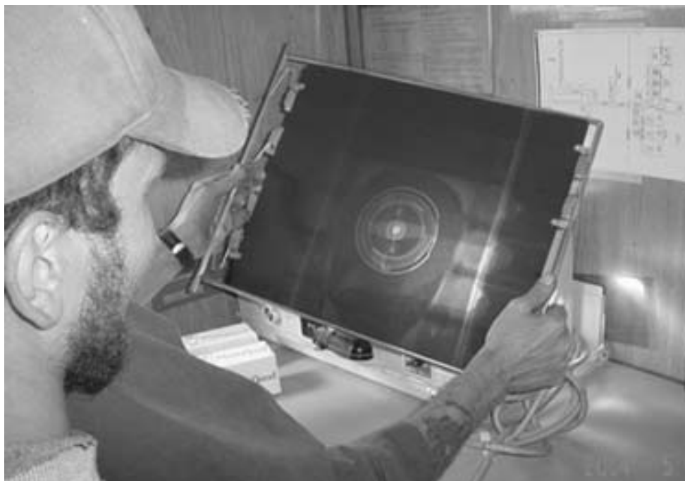
Left: Modern high-tech screening for a historic aircraft. An image reveals a rivet's structure.
