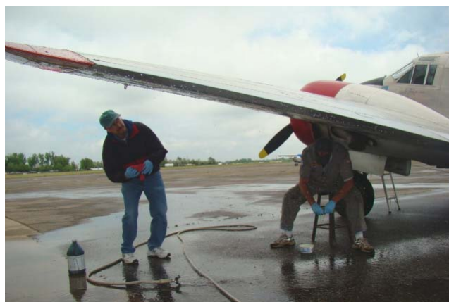
Col. Stan Hanson and Col. Mark Weigand wash and dry the left wing after cleaning it with Alodine.
