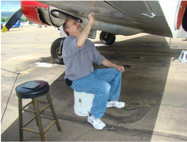
Col. Weigand cleans rivets before priming.
