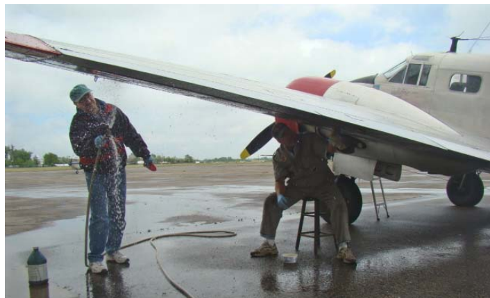
Col. Stan Hanson and Col. Mark Weigand wash and dry the left wing after cleaning it with Alodine.
