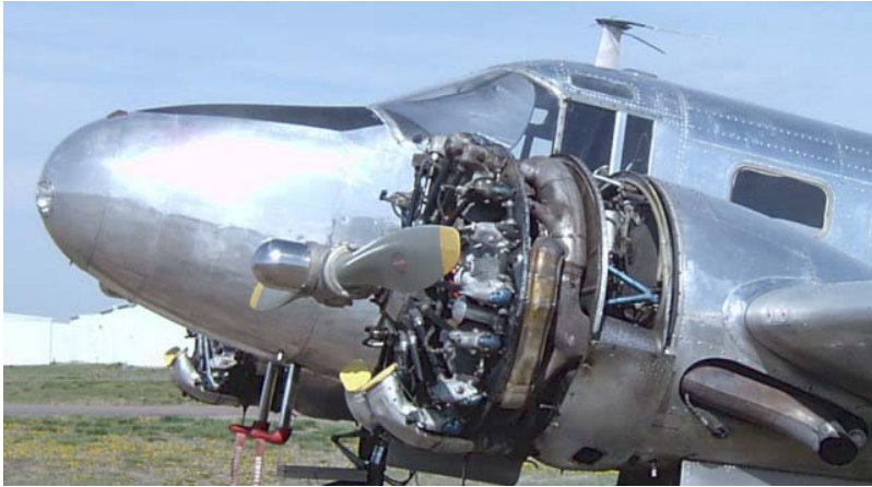
Above, engines with cowls removed before annual aircraft inspection.
