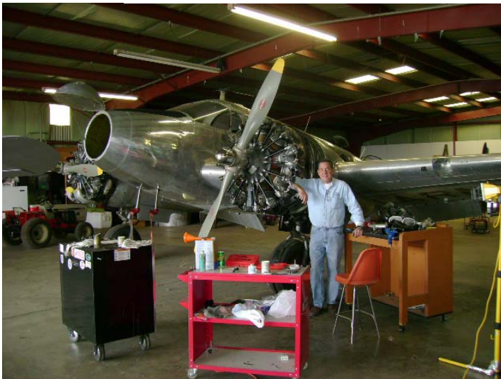
Above, engines with cowls removed before annual aircraft inspection.
