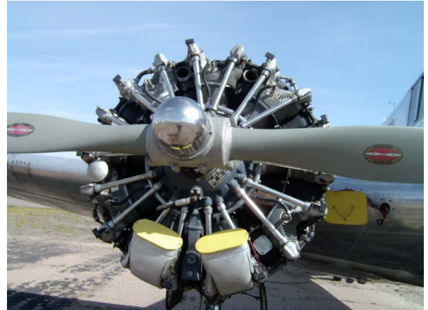
Above, engines with cowls removed before annual aircraft inspection.
